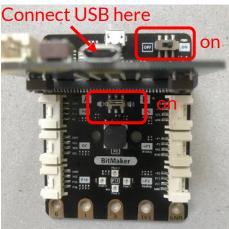
Plug the micro:bit into the BitMaker, setting both switches to "on".
