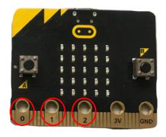
Challenge: The micro:bit and BitMaker expose pins 0, 1, and 2 on the bottom edge connector. "Say" the **analog** value of each pin while you touch it. Do the values change as you brush your finger over each pin?
