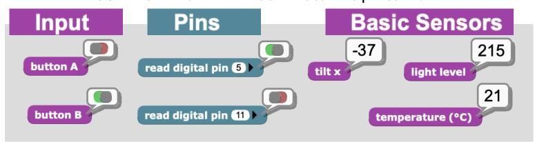
Use the "say" block in a forever loop to monitor various sensors. (Only run one forever loop at a time, or add all sensors into one "say" block.)
