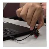
Figure 4: Tilting micro:bit on Challenge 1
