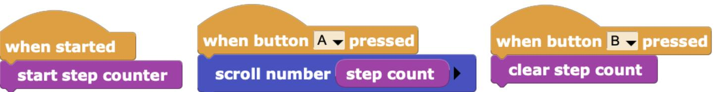
Now, plug in a battery and take your micro:bit for a walk! How well does it work? Reset the count, then take 20 steps. What count did you get? Adjust the sensitivity (lower if you are smaller) using this block.
